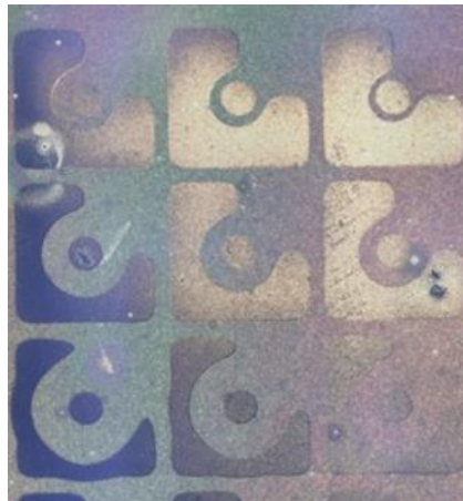
Figure 1. Sample for electrical property measurement of the acceptor-doped r\text{-GeO}_2 thin film
